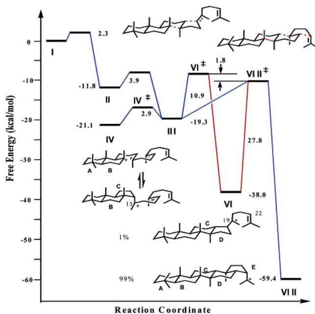
**Figure 8.** Relative free energies for key reaction intermediates and transition states in the mechanism of squalene cyclization (Scheme 4) in squalene–hopene cyclase. The minimum connected by red lines is proposed as a thermodynamic trap, leading to the 1% observed side products.
